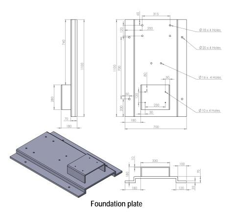
2. Drill and insert M20 anchor bolts to the concrete for mounting the foundation plate. Use grouting compound for securing anchor bolts to the concrete.
