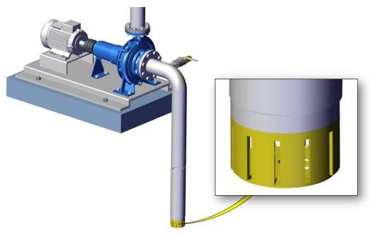
Non-return check valve at the bottom of the inlet pipe
