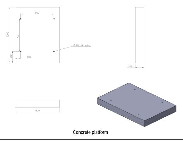
Construct a concrete platform of 1200 X 800 X 160 mm adjacent to the water pick-up point. Ensure the platform capacity ≥ 250 kgs. Level the platform to ± 1 mm. See <u>"Concrete platform" on page 9</u>.
