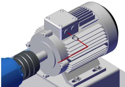
Wiring the motor through cable gland
